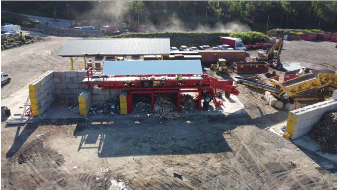
Michael Brothers uses a Keystrack Mobile Screen to segregate materials over four inches at its facility. Photo by Boyd Jones.
