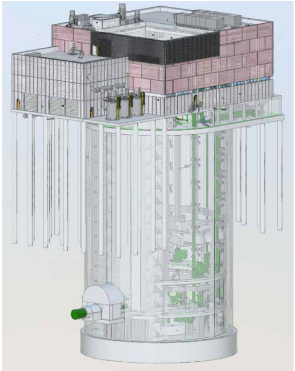
Rendering of the southeast façade and underground facilities of ALCOSAN's $200 million wet weather pump station, which will bid during the first quarter of 2025. Rendering by Brown and Caldwell. Use courtesy ALCOSAN.
